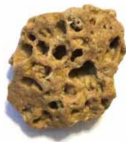
Secondary porosity caused by dissolution is visible in this rock specimen. Photo courtesy Michael Schnieders, PG, PH-GW, Water Systems Engineering Inc.
